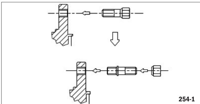
The wheel nuts may be changed, provided that their material remains ferrous. Alternatively, another method of retaining the wheels attachment system may be used provided it has been approved and homologated.
