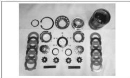
W1-5) Differential assembly on crown wheel
