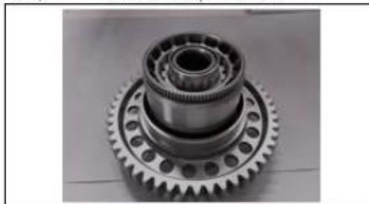
W1-5) Differential assembly on crown wheel
