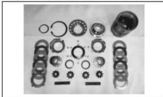
W1-5) Differential assembly on crown wheel
